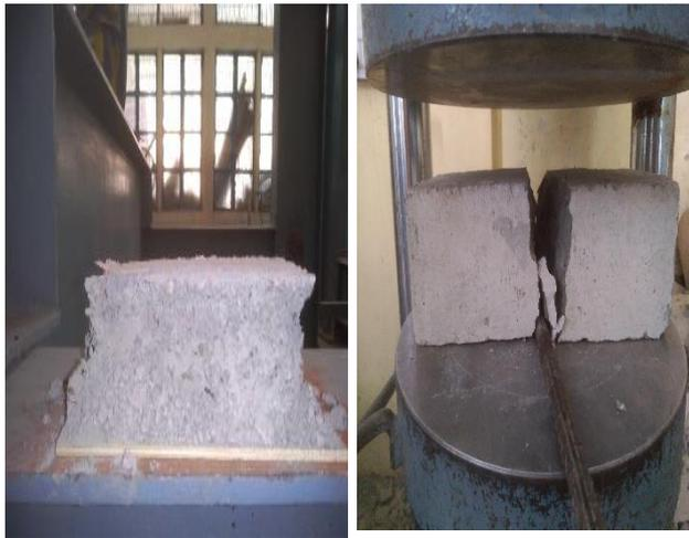
**Fig. 1.1** Compressive and tensile test of concrete brick unit.
