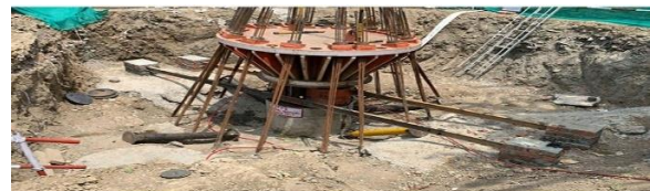
Fig. 8. Pile load testing setup at a construction site, featuring a reaction frame, tensioning rods, and hydraulic jacks to assess foundation strength and stability
