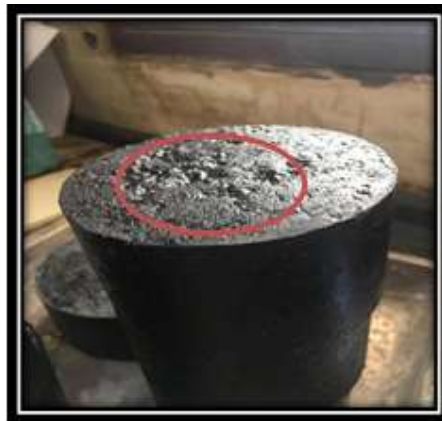
Figure(8): Raveling in MA specimen's surface.
